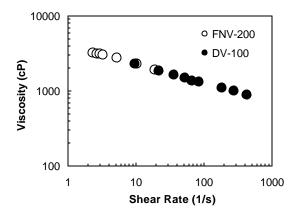
Viscosity measured by using the disposable viscometer (DV-100) compared to the data measured by the falling needle viscometer (FNV-200) for ointment at 25°C
