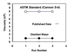
Viscosity measured by using the disposable viscometer (DV-100) compared to ASTM standard (Cannon S-6) and distilled water at 25°C
