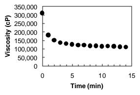
Fresh (0 min) vs. disturbed caulking viscosity measured every minute by using the caulking viscometer (CV-100) at 22.8°C
