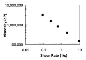
Viscosity measured by using the caulking viscometer (CV-100) for a caulking at 24.2°C
