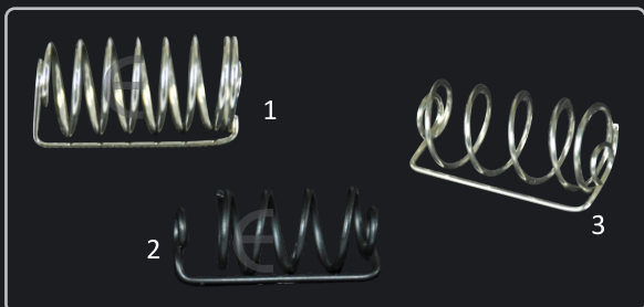
1. Helical coil sinker (L 2.4 cm D 0.1 cm & GAPS 0.5 cm) 2. Helical coil sinker – Capwht-02 3. Helical coil sinker – Capwht-2S
