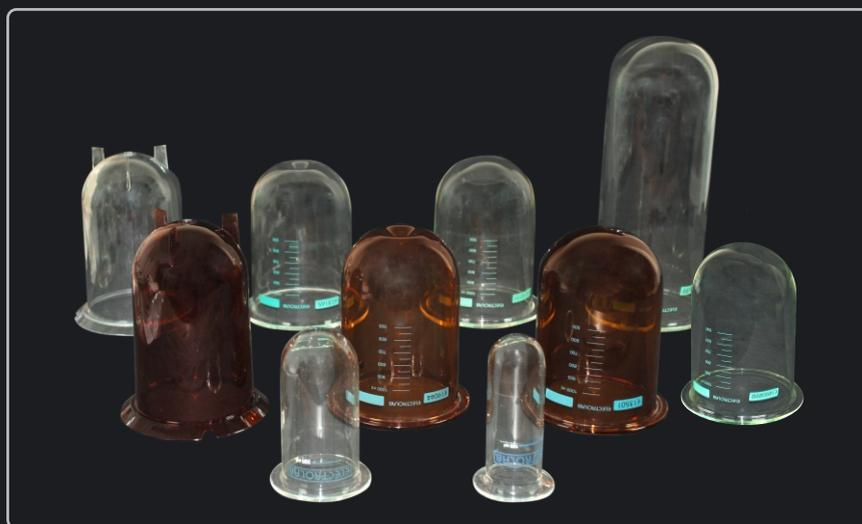
Dissolution test vessels in glass 100 ml, 250 ml, 1 ltr, 4 ltr capacity and Polycarbonate vessels in 1 ltr capacity. All the above are available in both clear and amber color
