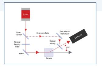
The electrophoretic velocity or movement of the particle is determined by using a laser light source and measuring scattered light with the APD positioned at a 15° scattering angle. This signal along with a reference signal are then optically mixed to determine the electrophoretic velocity.
