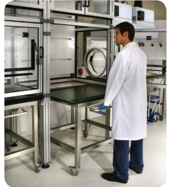
Carts are removable for cleaning and servicing of equipment. Additional carts were provided to allow for more than one piece of equipment to be placed in each enclosure.
